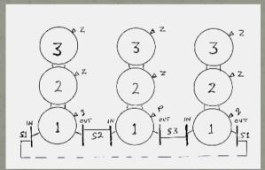
Loop condition satisfied if a voltage applied at some input L3 on left comes out at L3 on right -> no voltage on other 25 wires.
