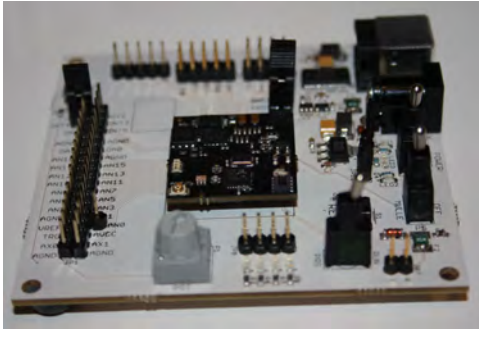
Fig. 3: Mulle v6.2 (black) on development board (white)
